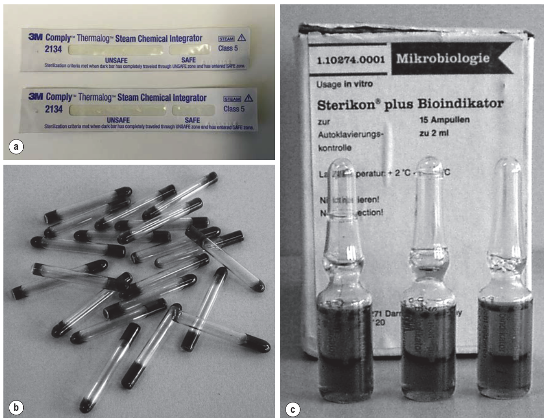
Fig. 17.5 Examples of chemical and biological indicators. (a) Multiparameter (time, steam and temperature) indicators. (b) Sterilization control tubes. (c) Geobacillus stearothermophilus biological indicators.
